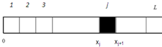
Fig. 1. J^{\text{th}} damaged element in beam.
