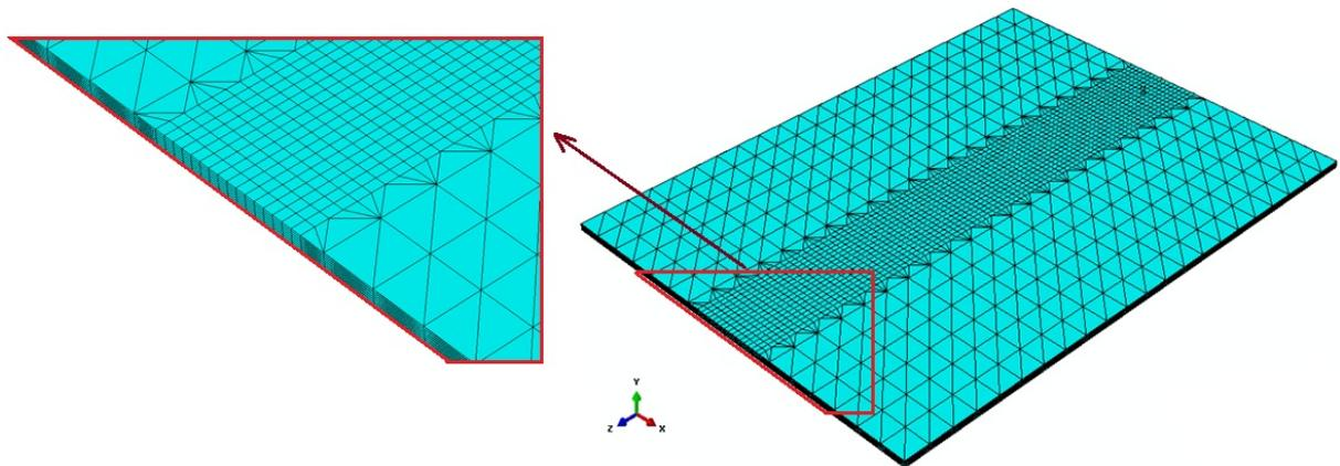
Fig. 4. Workpiece Meshing.
