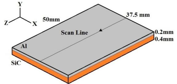
Fig. 2. Scheme of cermet piece.
