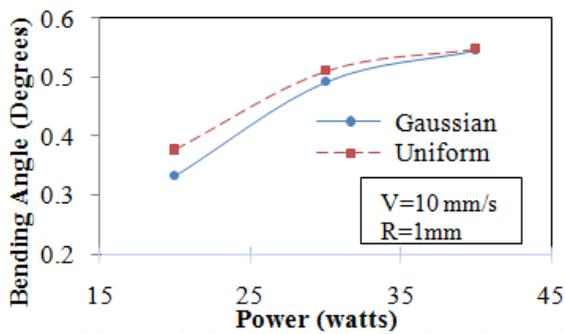
Fig. 9. Changes in bending angle for Gaussian and Uniform distribution of laser heat flux in different laser powers.
