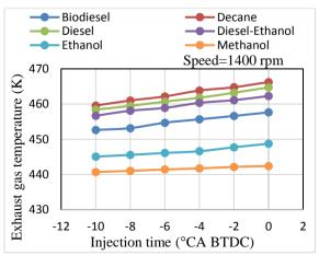
Fig. 7. Exhaust gas temperature at different injection timing.
