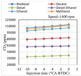
**Fig. 11.** CO<sub>2</sub> emission at different injection timing.
