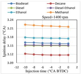
Fig. 4. Ignition delay at different injection timing.
