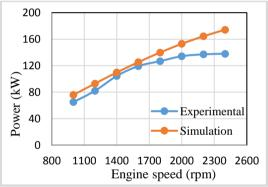
**Fig. 2.** Curve of engine power versus engine speed (comparison of experimental and simulation data) [22].
