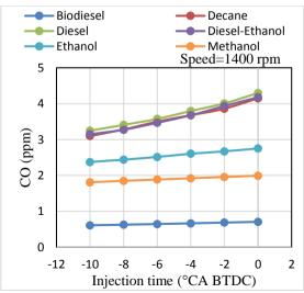
Fig. 9. CO emission at different injection timing.
