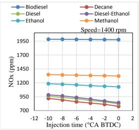
Fig. 12. NO<sub>X</sub> emission at different injection timing.
