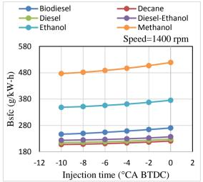
**Fig. 8.** Brake specific fuel consumption at different injection timing.
