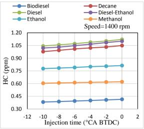
Fig. 10. HC emission at different injection timing.
