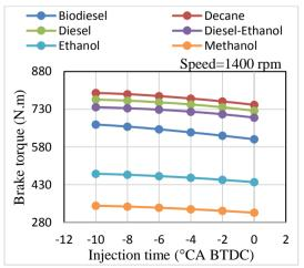
Fig. 6. Brake torque at different injection timing.
