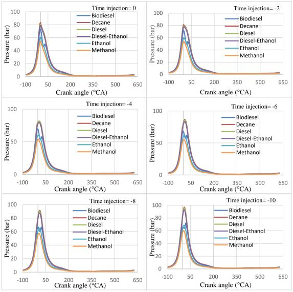
Fig. 5. Pressure in cylinder at different injection timing.
