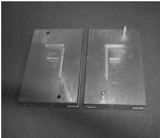
**Fig. 2.** An aluminum die used to produce wax patterns under different conditions.
