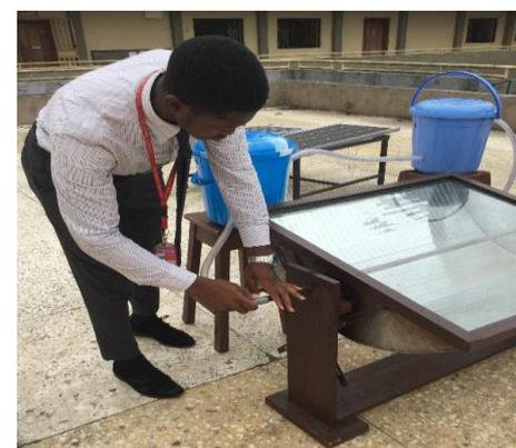
**Fig. 2.** Mini-parabolic solar concentrator with water storage tanks.
