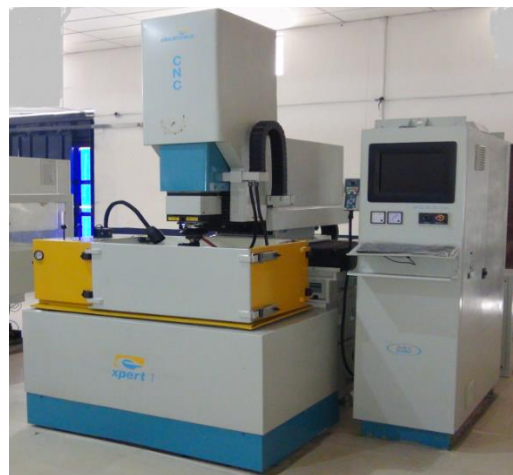
Fig. 1. Electronica make sinker EDM machine.
