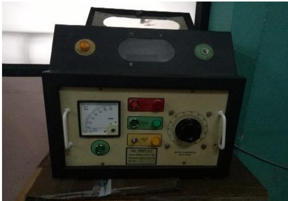
Fig. 4. Liquid dielectric test apparatus for breakdown measurement.
