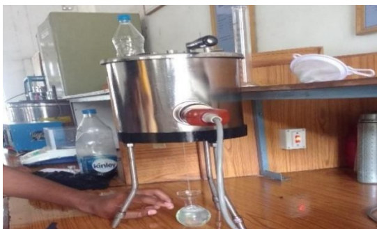
Fig. 7. Saybolt viscometer apparatus while conducting experimentation.
