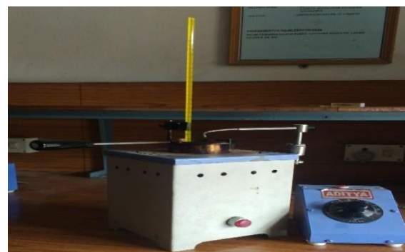
Fig. 8. Cleaveland flash & fire point apparatus during conducting of experimentation.
