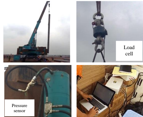
Fig. 19. The installation position of the load cell and the pressure sensors on the machine.
