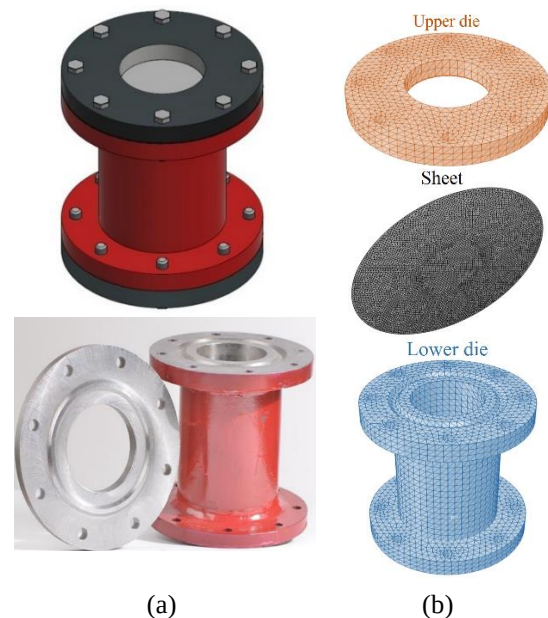
Fig. 2. (a) Designed and manufactured die and (b) meshing of the sheet and die.
