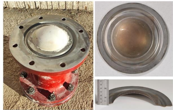
Fig. 3. Forming process by SCDA and the produced sample.
