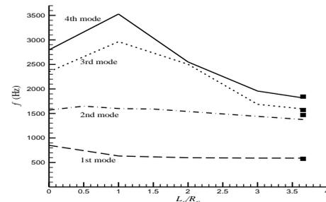
**Fig. 5.** Effect of cylinder length on the natural frequencies (Hz) of the structure for free-free boundary condition (solid squares are the experiment results).
