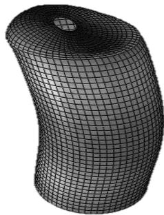
**Fig. 14.** Mode shape change in lower values of torispherical head depth.
