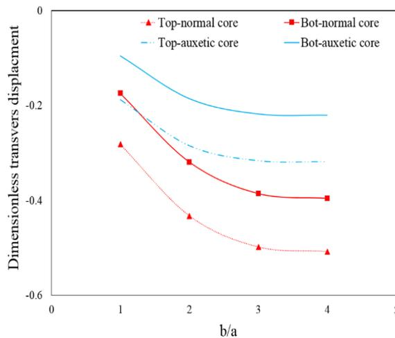
**Fig. 13.** The effect of the length-to-width ratio of the plate on the dimensionless transvers displacement of the middle points of the upper and lower surfaces belonging to the thick sandwich plate ( $a/h=4$ ) with a very soft core ( $E_f/E_c=10^5$ ) ordinary ( $\nu = +0.3$ ) and Auxetic ( $\nu = -0.5$ ).
