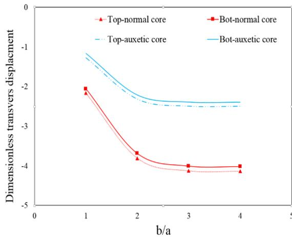
**Fig. 12.** The effect of the length-to-width ratio of the plate on the dimensionless transvers displacement of the middle points of the upper and lower surfaces belonging to the thick sandwich plate ( $a/h=4$ ) with a stiff core ( $E_f/E_c=10$ ) ordinary ( $\nu = +0.3$ ) and Auxetic ( $\nu = -0.5$ ).
