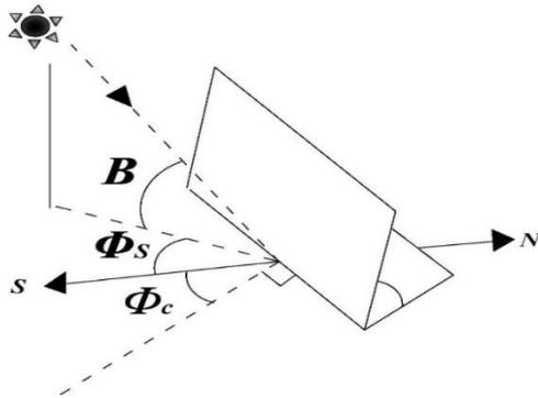
**Fig. 6.**  $\Phi_c$ : panel angle with south,  $\Phi_s$ : sun angle image with south and  $\Sigma$  : panel angle with the horizon.
