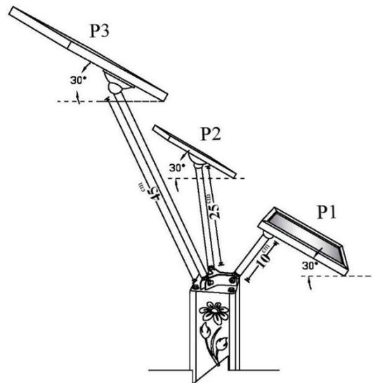
**Fig. 13.** The proper placements of panels on tree
