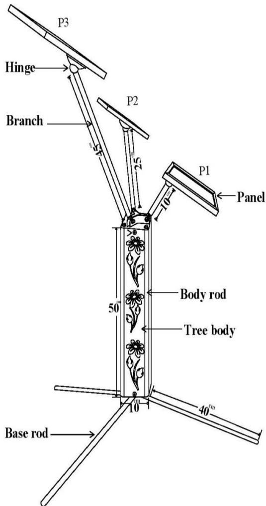
**Fig. 3.** The solar tree made according to the Fibonacci pattern
