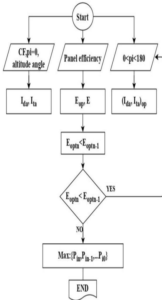
**Fig. 7.** The flowchart of optimized slope and maximum received energy calculation process
