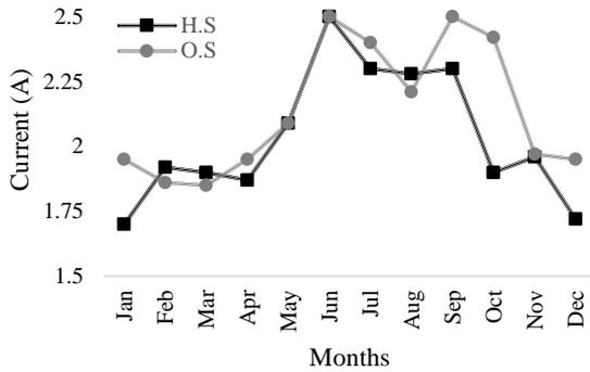
**Fig. 11.** Comparison of the received current at two fixed and optimal angles
