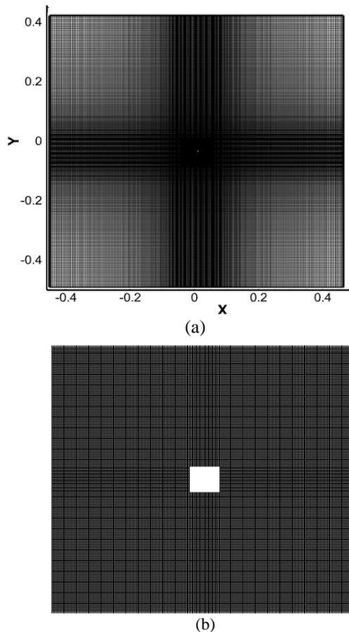
**Fig. 2.** Mesh of the computational domain; (a) Mesh structure for the full computational domain and (b) computational grid close to cylinder.
