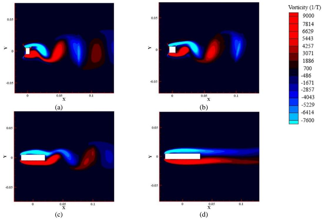
**Fig. 9.** Instantaneous vorticity ( $\omega_z$ ) contours in the near wake. The red contour indicate that the positive vorticity contours (counter-clockwise) and the blue contour indicate the negative vorticity contours (clockwise); (a)  $R = 0.6$ , (b)  $R = 1$ , (c)  $R = 4$ , and (d)  $R = 6$ .
