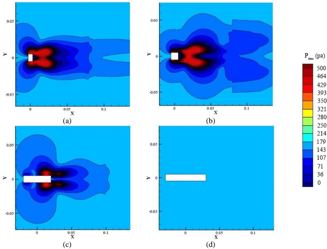
**Fig. 10.** Contour of root mean square pressure in different aspect ratio; (a)  $R = 0.6$ , (b)  $R = 1$ , (c)  $R = 4$ , and (d)  $R = 6$ .
