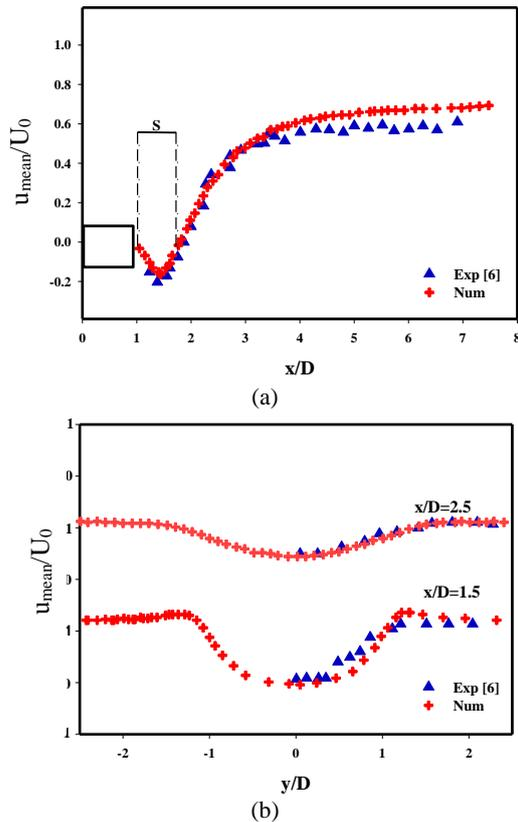
**Fig. 3.** Distribution of mean velocity in streamwise and spanwise direction comparing to experimental [6]; (a) streamwise mean velocity on centerline and (b) mean velocity at two streamwise locations.
