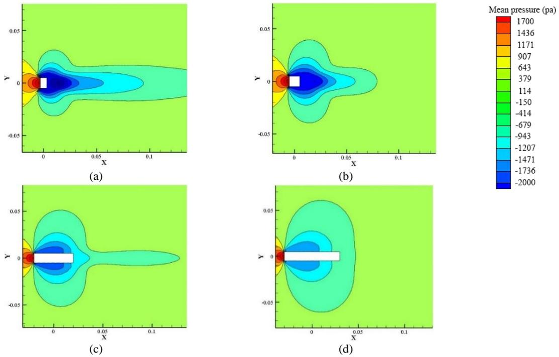
**Fig. 8.** Mean static pressure contours in different cases of rectangular cylinder; (a)  $R = 0.6$ , (b)  $R = 1$ , (c)  $R = 4$ , and (d)  $R = 6$ .
