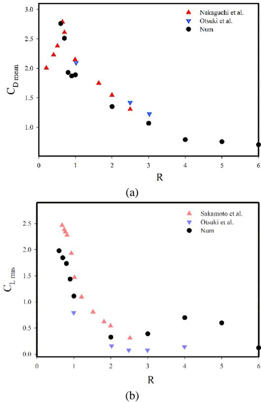
**Fig. 7.** Variations of aerodynamic characteristics for different aspect ratios (Nakaguchi *et al.* [12], Otsuki *et al.* [28], Sakamoto *et al.* [29]); (a) average values of the drag and (b) root mean square of the lift coefficient.
