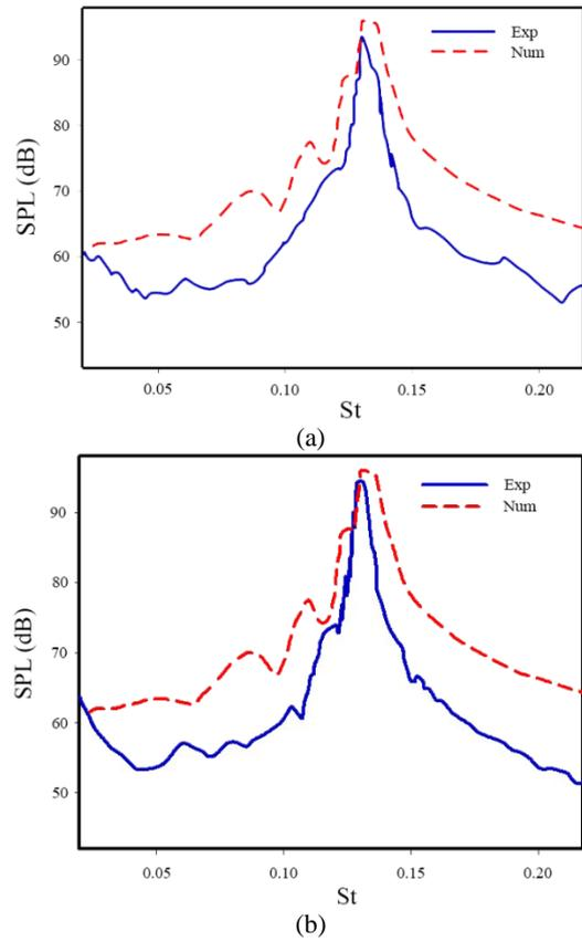
**Fig. 4.** Numerical and experimental [27] acoustic SPL versus St; (a) microphone (1) and (b) microphone (2)
