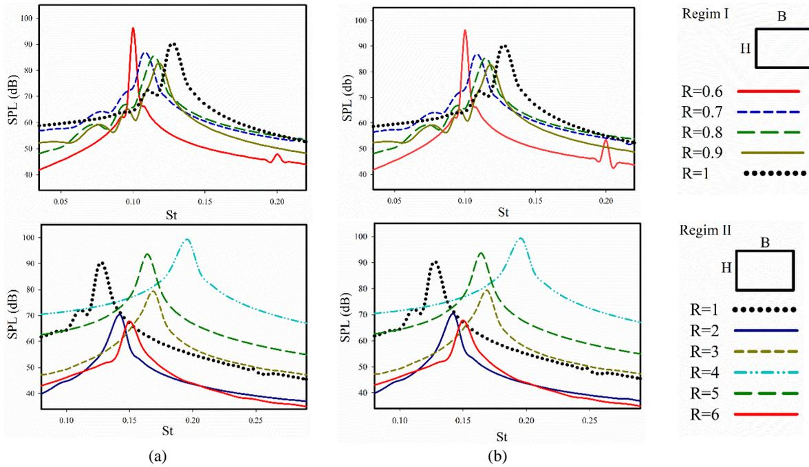
**Fig. 5.** Sound pressure level a rectangular cylinder with different aspect ratios; (a) microphone (1) and (b) microphone (2).
