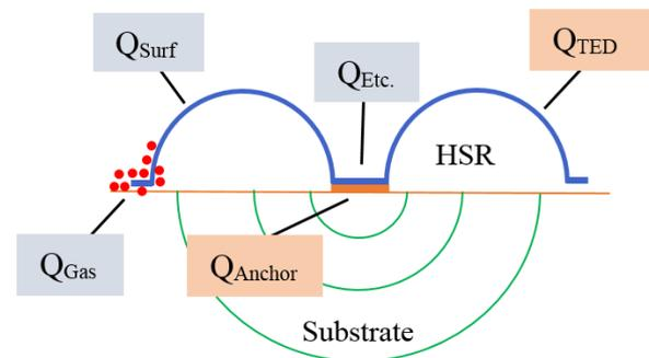
**Fig. 3.** Showing various energy loss factors in a HSR with a mushroom structure.
