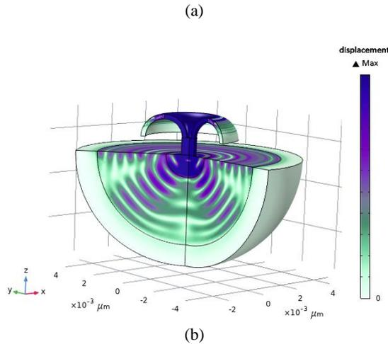
**Fig. 8.** Two-dimensional and three-dimensional simulation of anchor loss in COMSOL software. (a) Two-dimensional design of the shell and PML region. (b) Three-dimensional view of anchor loss and energy escape from the shell to the substrate.
