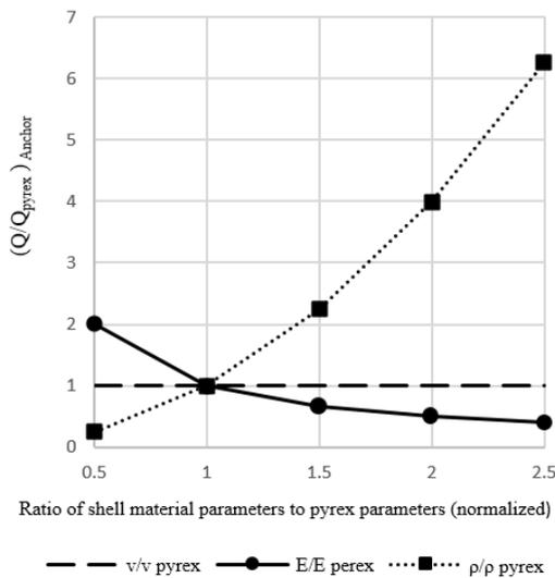
**Fig. 7.** Study of the effect of shell properties on anchor loss
