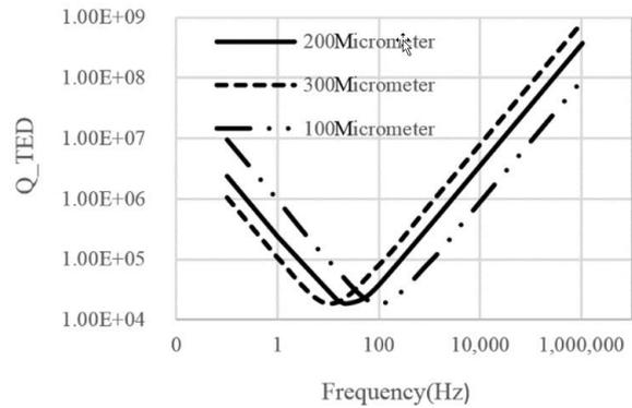
Fig. 4. Thermo-elastic dissipation curve in terms of resonance frequency
