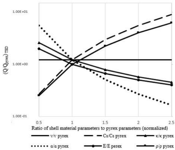
**Fig. 5.** Effect of shell material properties on thermo-elastic damping
