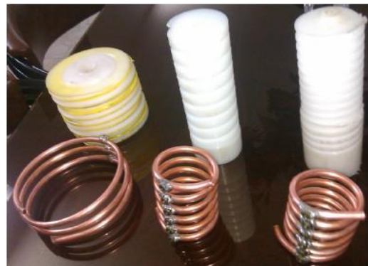
Fig. 2. Triple-tube helical heat exchanger with their Teflon module.
