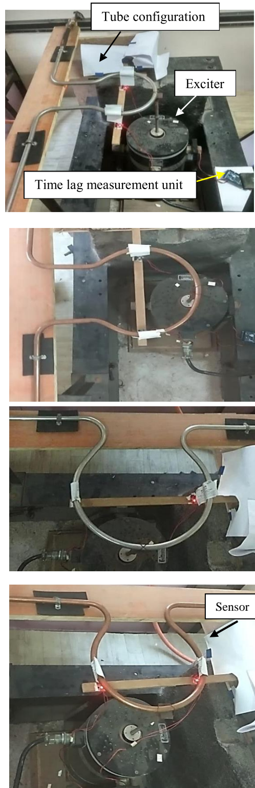
Fig. 5. Experimental set-up for the Omega models.
