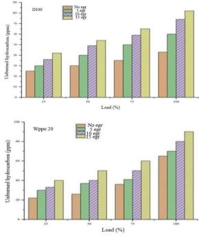
**Fig. 16.** UHC emissions from burning biodiesel as well as WPPO with different load and EGR percentages.
