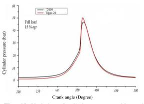
Fig. 10. Variation of cylinder pressure with crank angle.
