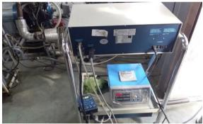
**Fig. 8.** Photo graphical view of avl 437 standard smoke meter.
