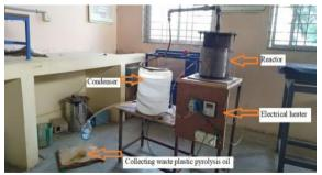
Fig. 2. Pyrolysis equipment.
