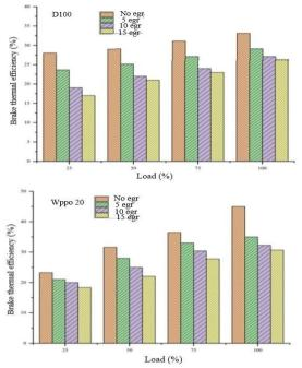
**Fig. 12.** BTE of diesel and WPPO biodiesel combustion at different load and EGR conditions.
