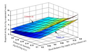
**Fig. 12.** Theoretical required air usage at various exhaust humidity and hood balance.
