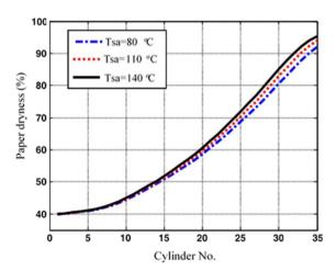
Fig. 16. Paper web dryness profile at various supply air temperature.
