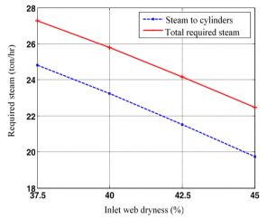
**Fig. 8.** Steam usage in drying section at various inlet web dryness.
