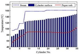
**Fig. 2.** Temperature variations of the paper web and cylinder surface (modeling results).
