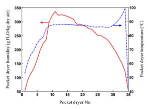
**Fig. 4.** Temperature and humidity variations of drying pocket dryers.
