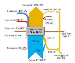
Fig. 17. Sankey diagram of studied drying section after optimization.
