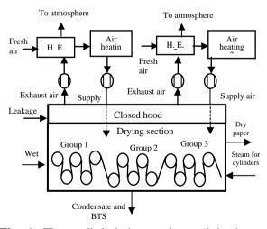
**Fig. 1.** The studied drying section and its heat recovery system.
