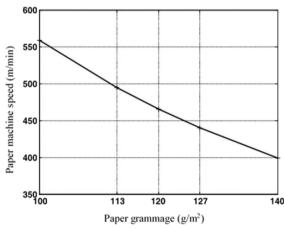
Fig. 6. Paper machine speed variation vs. paper grammage.
