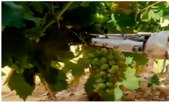
Fig. 4. The end-effector employed in agricultural robotics for fruit harvesting detaches fruits by gripping them from the stem and cutting [24].
