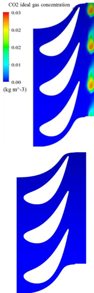
**Fig. 18.** Distribution of CO<sub>2</sub> concentration in a plane close to the hub: (a)  $\Phi_0 = 0.21$  and (b)  $\Phi_0 = 0.003$ .
