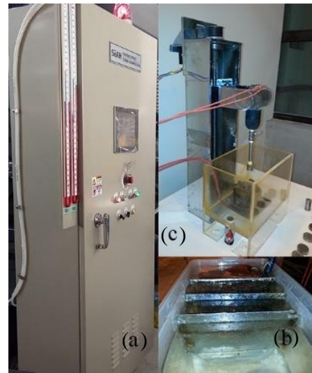
Fig. 2. Equipment for experiments: (a) power supply and control unit, (b) transmission and supply of electrolyte fluid unit, and (c) tool feeding unit.
