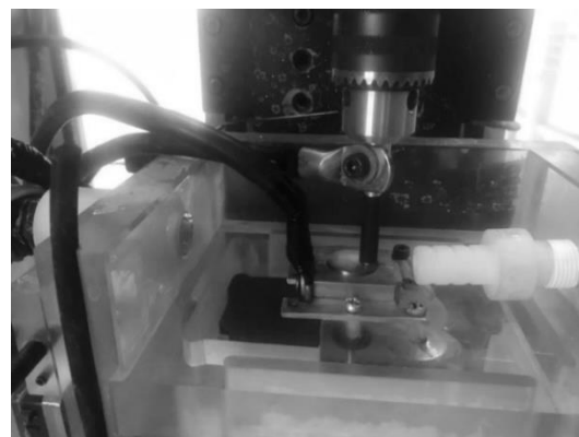
Fig. 2. Electrochemical machining chamber with tool and workpiece.
