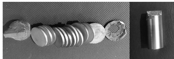
Fig. 1. CMSX-4 workpiece as heat treatment.
