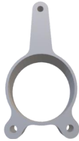
Fig. 15. Designed model of tendon guide.
