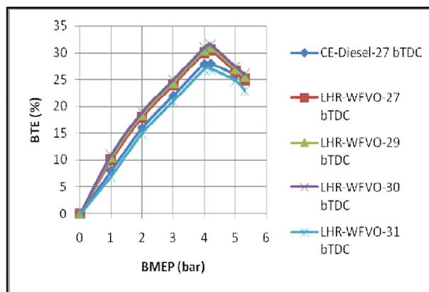
**Fig. 7.** Variation of brake thermal efficiency (BTE) with brake means effective pressure (BMEP) in engine with LHR combustion chamber at different injection timings with WFVO.
