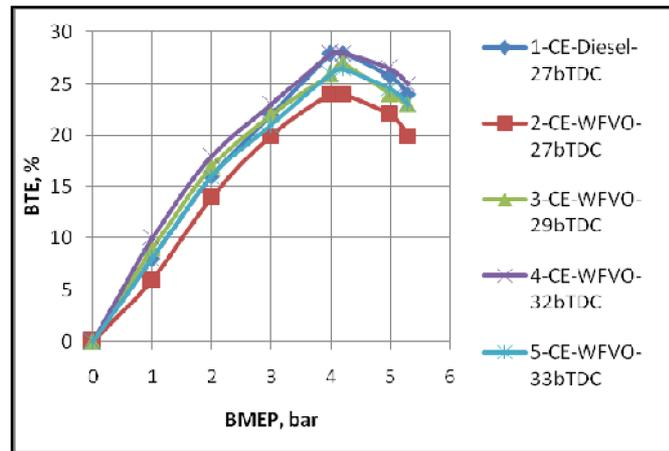
**Fig. 6.** Variation of brake thermal efficiency (BTE) with brake mean effective pressure (BMEP) in conventional engine (CE) at different injection timings with waste fried vegetable oil (WFVO) operation.
