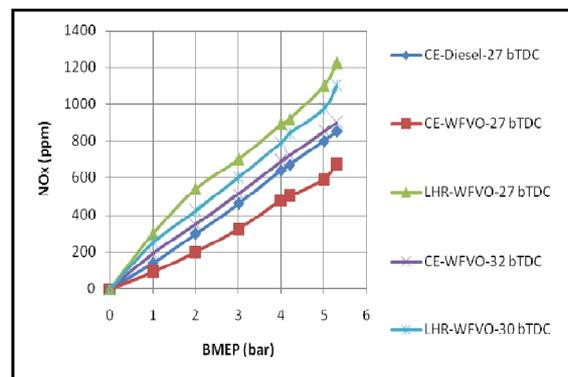
**Fig. 13.** Variation of nitrogen oxide levels (NO<sub>x</sub> levels) with brake mean effective pressure (BMEP) in the conventional engine and engine with LHR combustion chamber at the recommended injection timing and optimized injection timings with crude waste fried vegetable oil (WFVO) operation.
