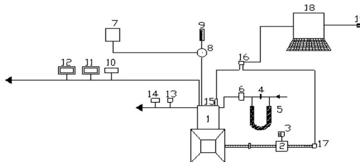
1. Engine, 2.Electical dynamometer, 3.Load box, 4.Orifice meter, 5.U-tube water manometer, 6.Air box, 7.Fuel tank, 8, Pre-heater, 9.Burette, 10. Exhaust gas temperature indicator, 11.AVL smoke meter, 12.Netel chromatograph NOx analyzer, 13.Outlet jacket water temperature indicator, 14. Outlet-jacket water flow meter, 15.Piezo electric pressure transducer, 16.Console, 17.TDC encoder, 18.Pentium personal computer and 19.Printer.
