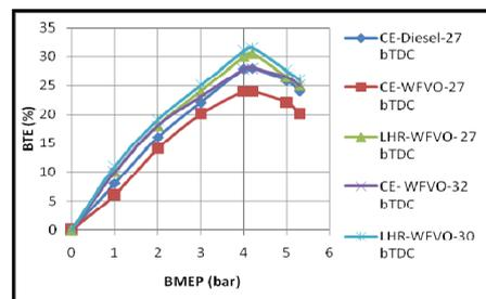
Fig. 8. Variation of brake thermal efficiency (BTE) with brake mean effective pressure (BMEP) with both versions of the combustion chamber at their optimum injection timings at the injector opening pressure of 190 bar.
