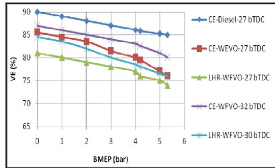
**Fig. 10.** Variation of volumetric efficiency (VE) with brake mean effective pressure (BMEP) in the conventional engine (CE) and engine with LHR combustion chamber at the recommended injection timing and optimized injection timings with waste fried vegetable oil (WFVO) operation.
