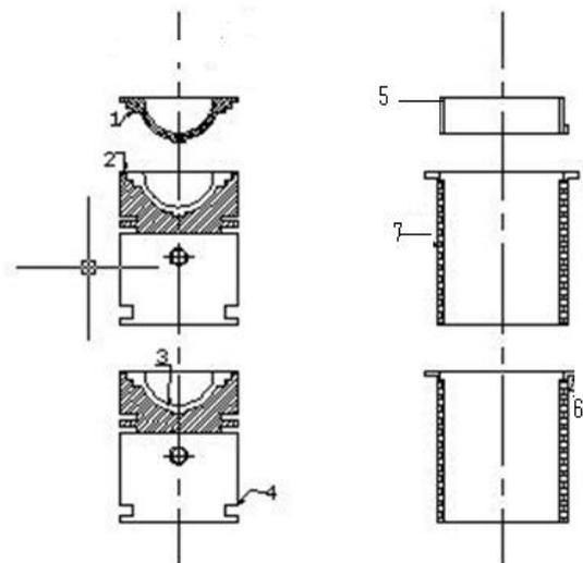
1. Superni crown, 2. Superni gasket, 3. Air gap in the piston, 4. Aluminium body of the piston, 5. Superniinsert, 6. Air gap in the liner, 7. Body of the liner.
