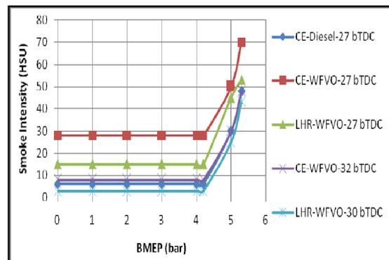
**Fig. 12.** Variation of smoke intensity in Hartridge smoke unit (HSU) with brake mean effective pressure (BMEP) in the conventional engine (CE) and engine with LHR combustion chamber at the recommended injection timing and optimized injection timings with crude WFVO.
