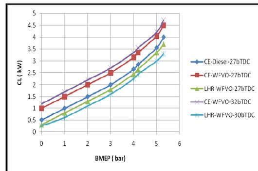
**Fig. 11.** Variation of coolant load (CL) with brake mean effective pressure (BMEP) in conventional engine (CE) and engine with LHR combustion chamber at the recommended injection timing and optimized injection timings with waste fried vegetable oil (WFVO) operation.
