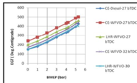
Fig. 9. Variation of exhaust gas temperature (EGT) with brake mean effective pressure (BMEP) in conventional engine (CE) and LHR engine at the recommended injection timing and optimized injection timings with waste fried vegetable oil (WFVO) operation.
