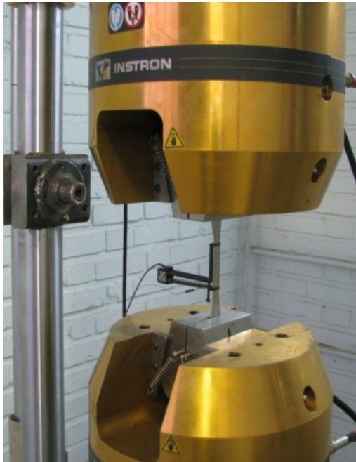
Fig. 6. Tension test by a servo hydraulic INSTRON 8802 machine.
