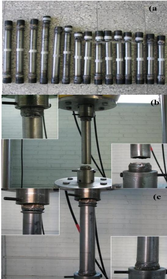
**Fig. 18.** a) A few numbers of tested cylindrical shells; b) failure of specimen near the welded spots; c) buckling of specimens near the welded fixtures.
