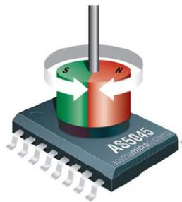
Fig. 1. Schematic of the magnet and the sensor [19].
