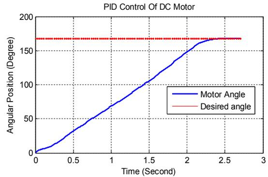
Fig. 6. Controlled DC motor using PID controller.
