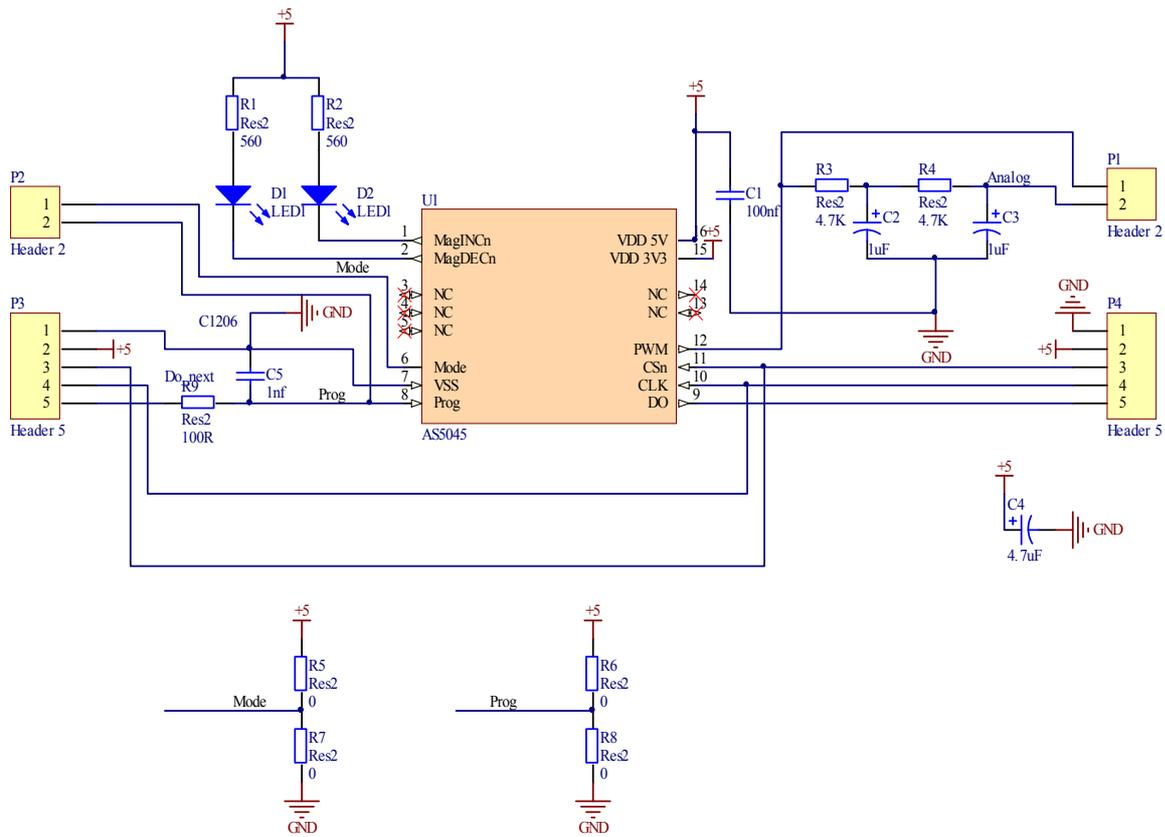
Fig. 3. Schematic of driver circuit of encoder.
