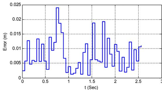
**Fig. 14.** Tracking end-effector error in circular path.
