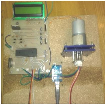
Fig. 4. Driver board mounted on a DC motor.
