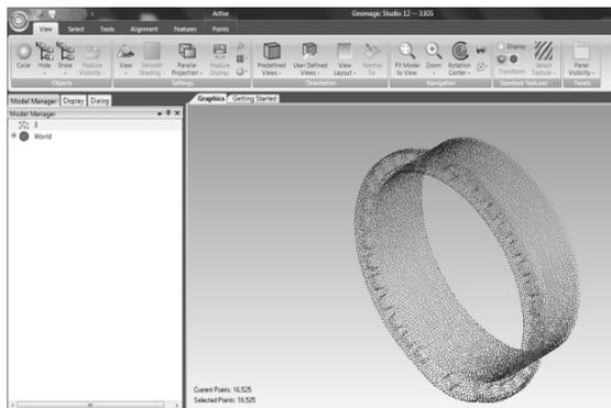
**Fig. 8.** 3D point cloud model of manufactured plastic bush.
