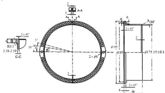
**Fig. 1.** Dimensions of the selected plastic bush (in millimeters).
