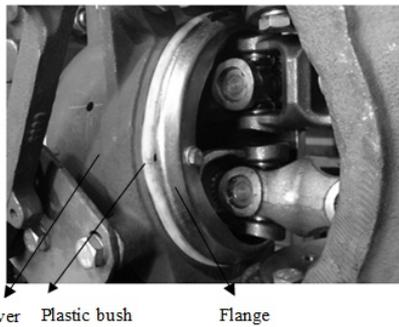
**Fig. 2.** Plastic bush assembled between cover and flange in the articulation central of the tractor.
