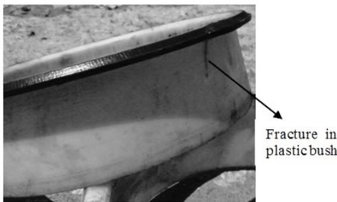
**Fig. 3.** Generated fracture in plastic polyethylene bush.
