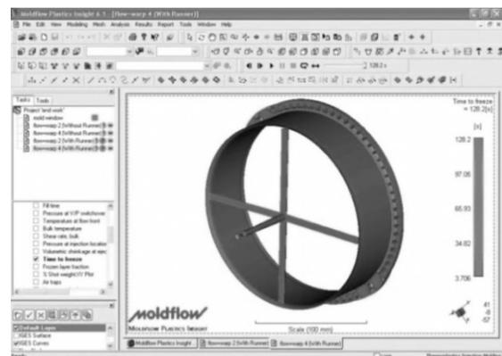
**Fig. 4.** Simulation of the injection molding process in Mold Flow software.
