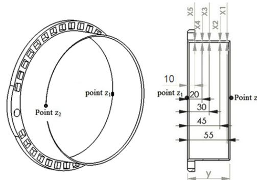
**Fig. 5.** Considered positions on the plastic bush geometry.
