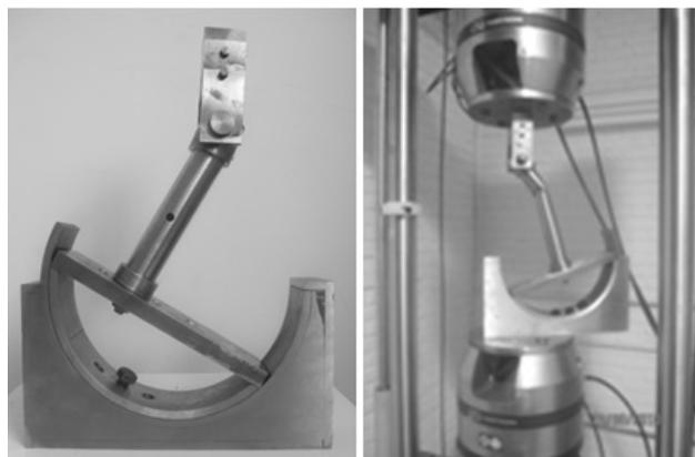
**Fig. 7.** INSTRON 8802 machine and designed fixtures.
