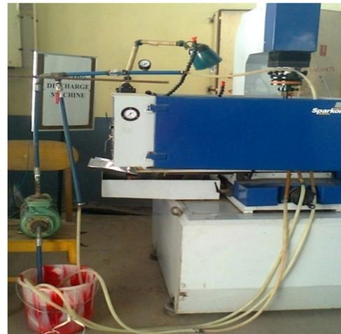
**Fig. 1.** Photographic representation of EDM system using separately developed de-ionized water circulating system.
