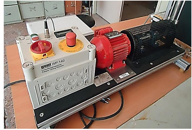
Fig. 4. Experimental equipment for rotating bending tests
