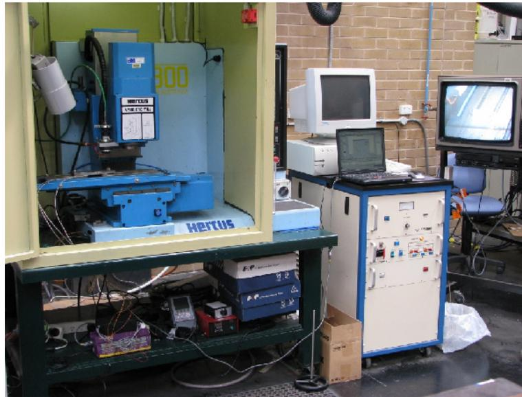
Fig. 2. The Nd:YAG laser rig with the X-Y table controller.
