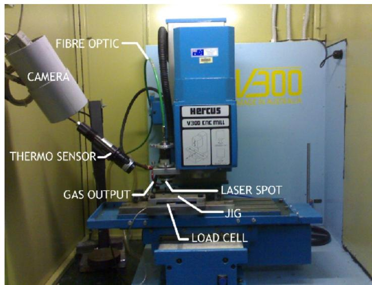
Fig. 3. The Jig, infrared device, and load cell location in the laser experimental rig.
