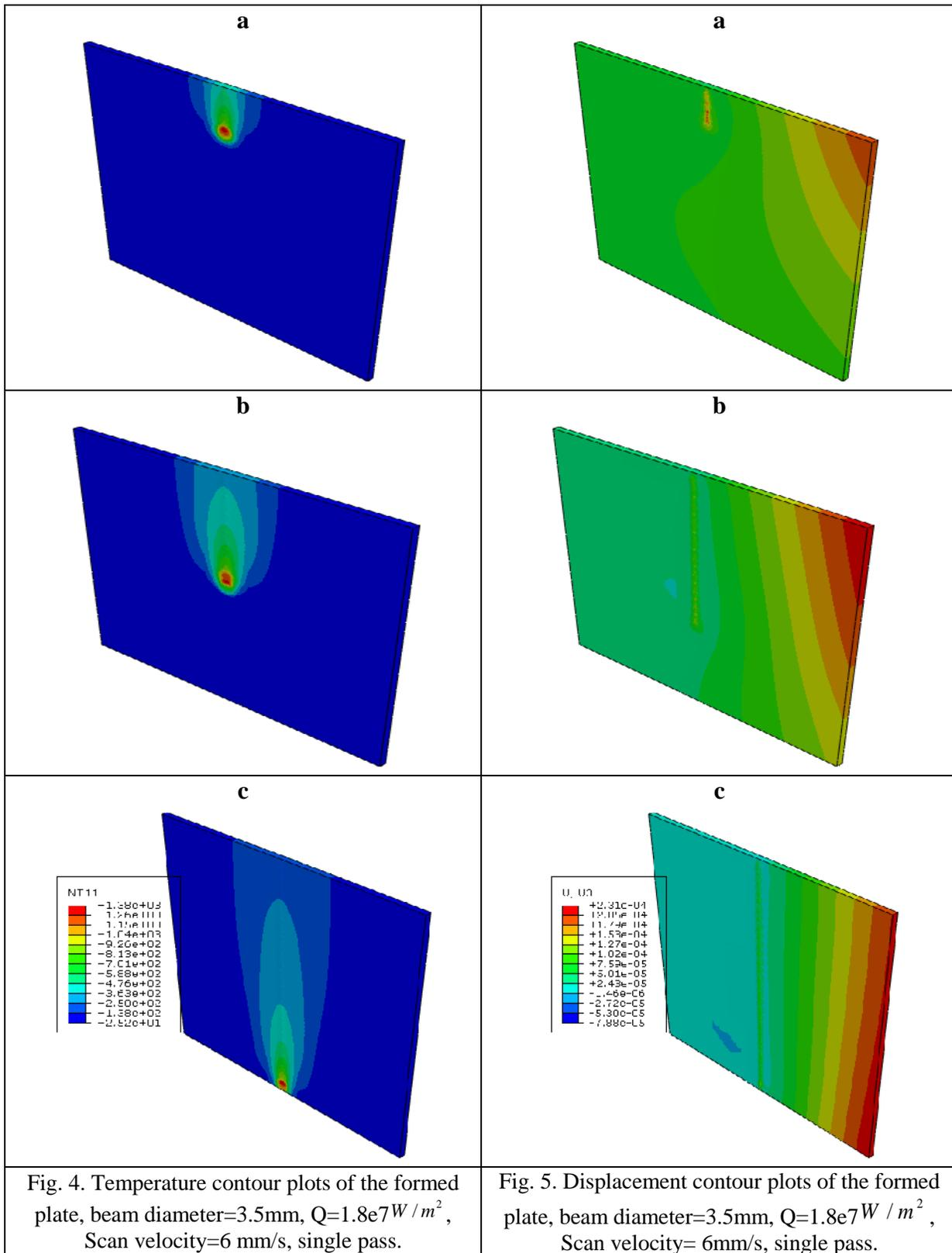
Fig. 4. Temperature contour plots of the formed plate, beam diameter=3.5mm,  $Q=1.8e7W / m^2$ , Scan velocity=6 mm/s, single pass.
