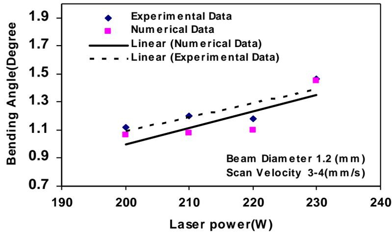
Fig. 6. Comparison between experimental and numerical results.
