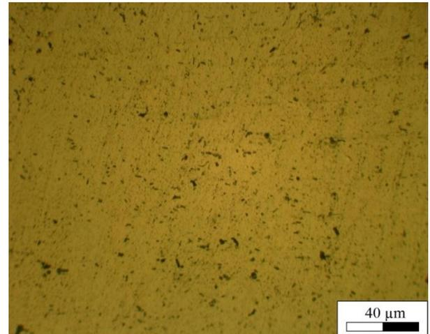
**Fig. 2.** Unwanted precipitates which are very fine and scares; specimen E2 (without aging).
