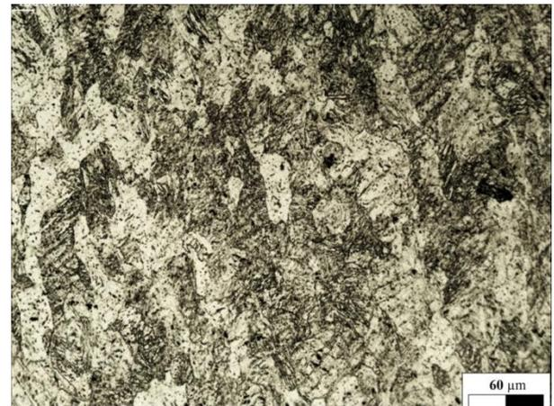
**Fig. 3.** Very fine and elongated grains resulted from ECAP; specimen E2.
