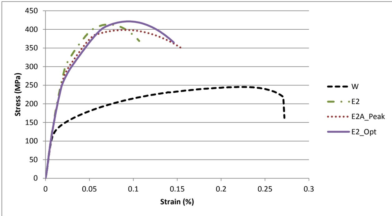
Fig. 8. Stress-strain curves obtained by conducting tensile tests on the specimens.
