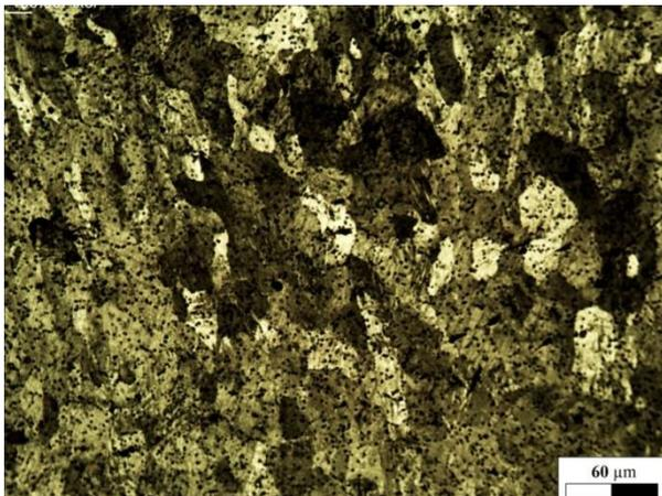
Fig. 5. Large precipitates along with recovered crystals as a result of peak aging, specimen E2A<sub>Peak</sub>.
