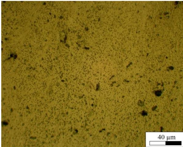
**Fig. 6.** Small size particles with high density and distribution in the matrix of alloy in E2<sub>Opt</sub> condition.
