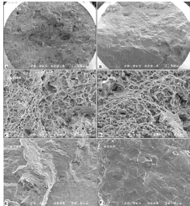
Fig. 10. Fatigue fractured surfaces of E2A<sub>Peak</sub> and E2<sub>Opt</sub> at the fatigue loading with the stress amplitude of respectively 318 and 337 MPa, and cycles to failure respectively 3640 and 6830. A: .
