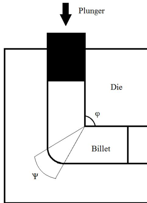
Fig. 1. Schematic of the ECAP process.
