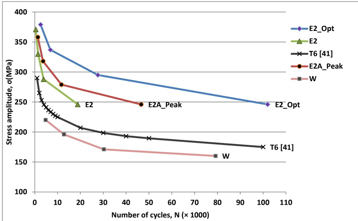
Fig. 9. S-N curves for the studied specimens; data of T6 extracted from [42] is embedded here for comparison purposes.
