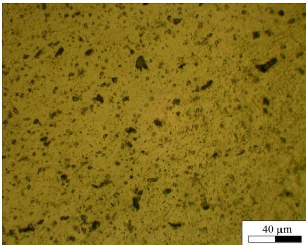
Fig. 4. Large and abundant precipitates in peak-aged UFG specimen, E2A<sub>Peak</sub>.
