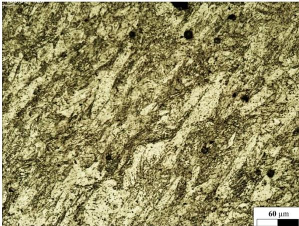
**Fig. 7.** Very distorted microstructure with large number of completely dispersed precipitates, E2A<sub>Opt</sub> condition.
