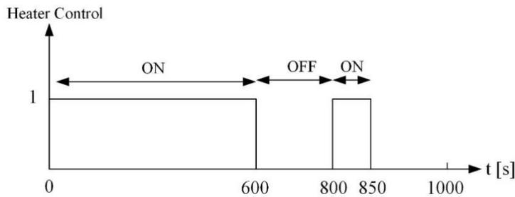
Fig. 7. Control method of heaters power.
