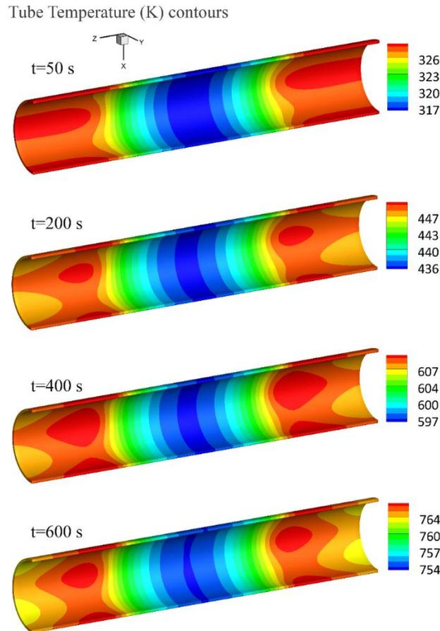
Fig. 6. Temperature contours of the tube surface.
