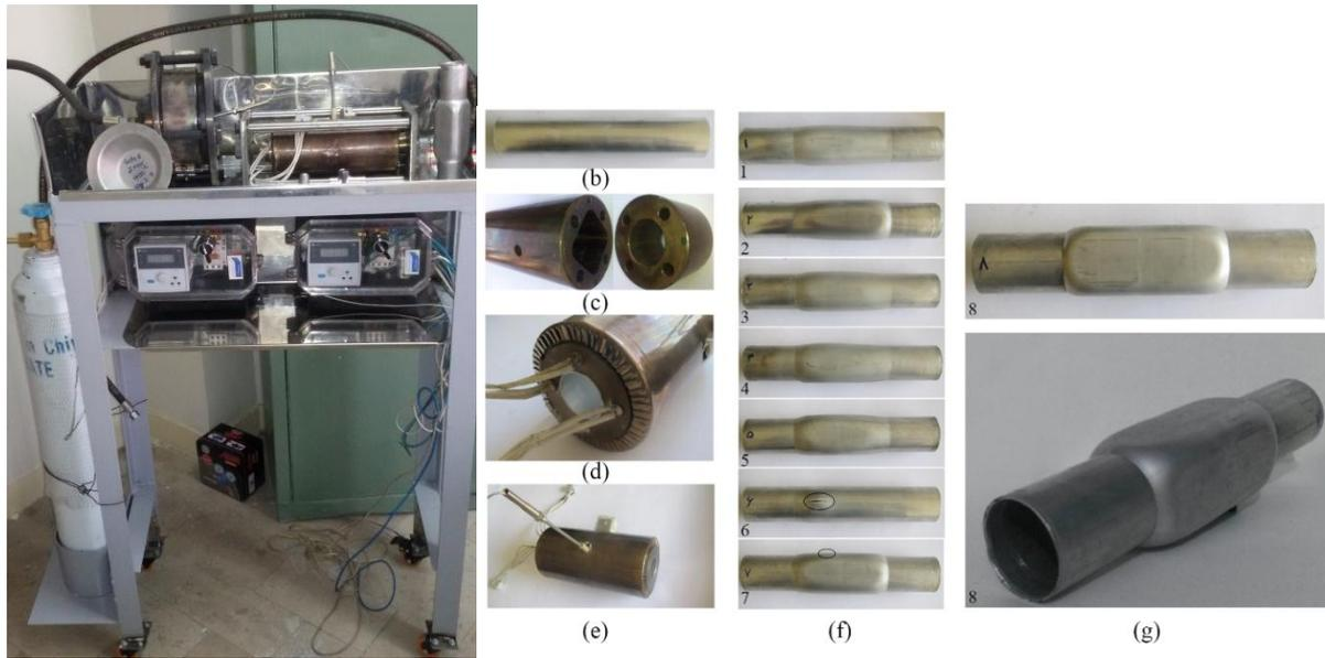
**Fig. 2.** Experimental setup (a) constructed setup (b) unformed tube (c) die (d) die and heaters (e) temperature sensor location (f) unsuccessful forming attempts (g) satisfactory forming.
