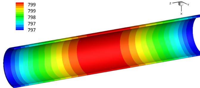
**Fig. 8.** Contour of tube temperature at  $t=1000$  s by applying the heater power control method.
