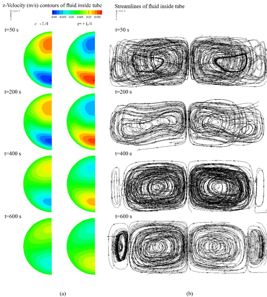
**Fig. 4.** (a) Contours of z-velocity at various z-planes (b) streamline of fluid inside the tube, at different times from the beginning.
