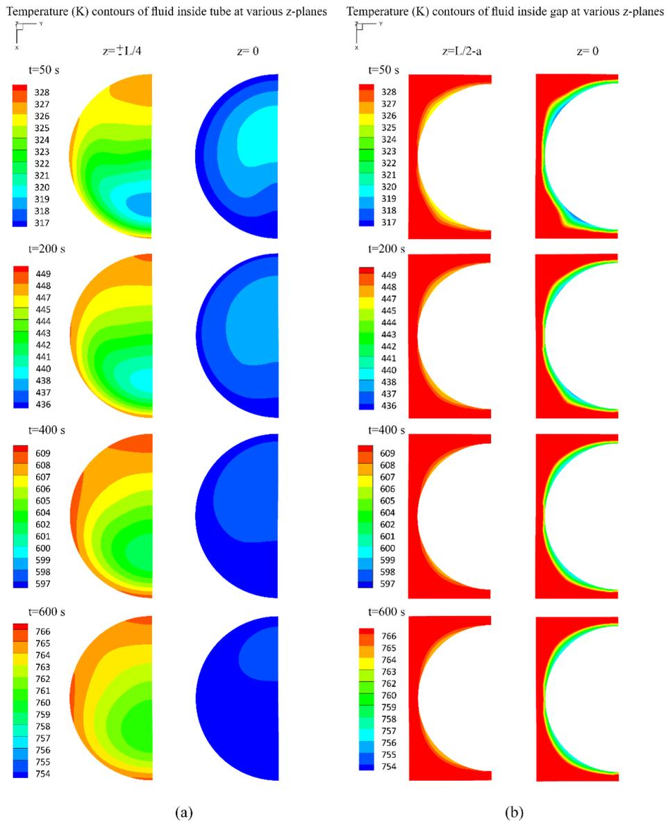
**Fig. 5.** Temperature Contours (a) fluid inside the tube (b) fluid trapped between the tube and die at various z-planes and different times from the beginning.
