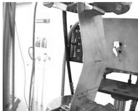
Fig. 6. Condition of applying axial compression load to the specimens using INSTRON machine.
