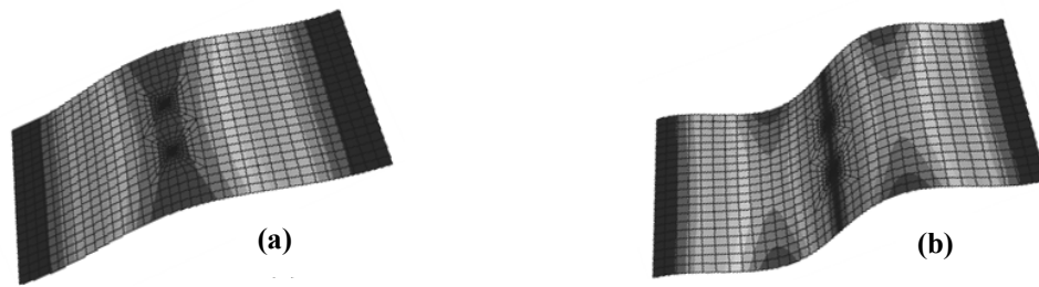
Fig. 8. Mode shapes of CC-200-100-0.2-4-0 specimen (a) first mode shape, and (b) second mode shape.
