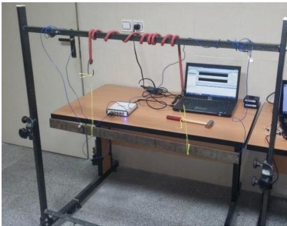
Fig. 2. Setup of OMA test.
