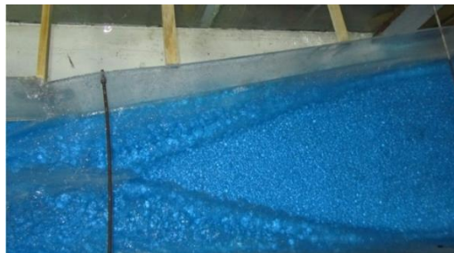
Fig. 2. Formation of the shock waves in the model 1 for Fr_1 = 7.0 .
