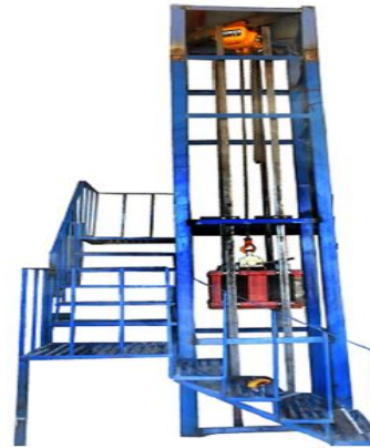
Fig. 3. Schematic of the free-fall drop hammer.
