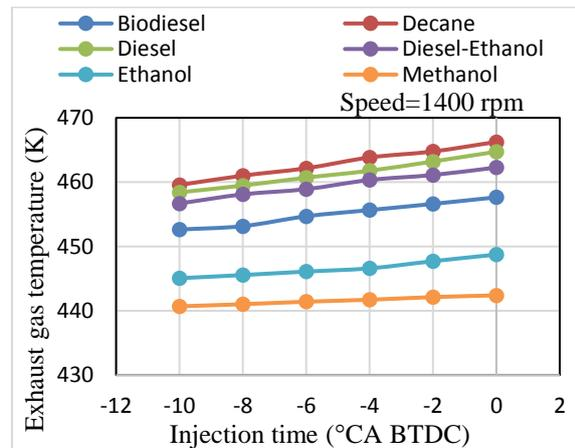
Fig. 7. Exhaust gas temperature at different injection timing.
