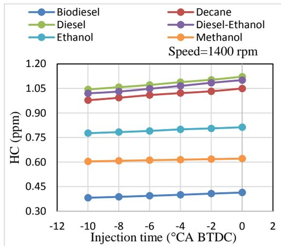
Fig. 10. HC emission at different injection timing.
