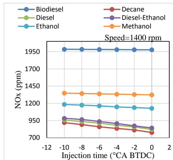
Fig. 12. NO<sub>x</sub> emission at different injection timing.
