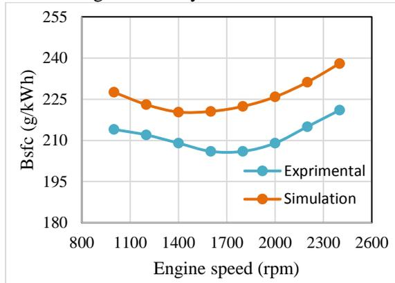
**Fig. 3.** Curve of brake specific fuel consumption versus engine speed (comparison of experimental and simulation data) [22].
